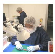
Precision Associates' medical grade products are produced and packaged in our ISO 14644-1 Class 7 certified clean room. Although manufacture takes place in a clean room, it is not a sterile environment. Precision Associates medical grade materials may be sterilized by EtO, autoclave or gamma radiation.
